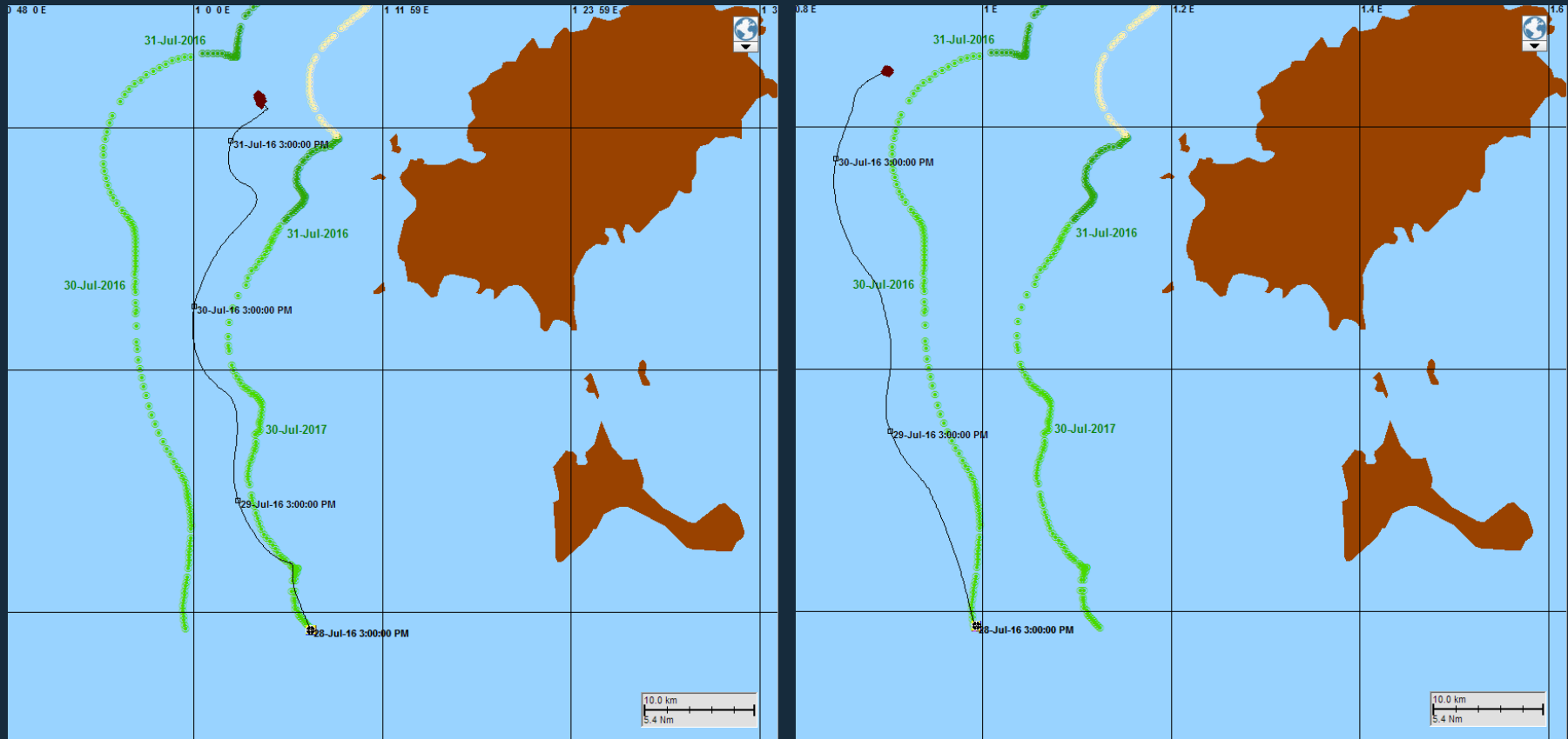
OILMAP viewer: Oil spill trajectory (using HFR currents) –black- vs. real drifters trajectories –colored-
